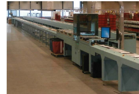
Below and left: The Dispatcher Max key features include sorting bins with bin full detection and LED display, delay module with 0-30 second delay configuration and multiple OCR and overseas video encoding
