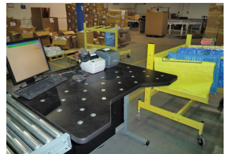
M-Bag bagging station and bag rack
