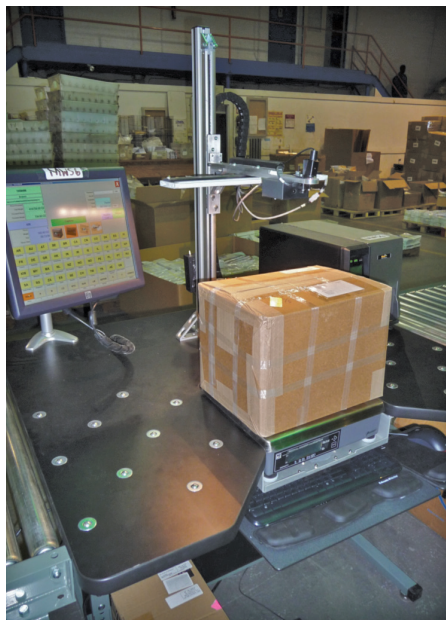
MMW station with imaging camera system
