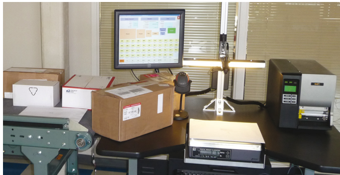
Enhanced MMW station for electronic data capture with new OCR imaging
