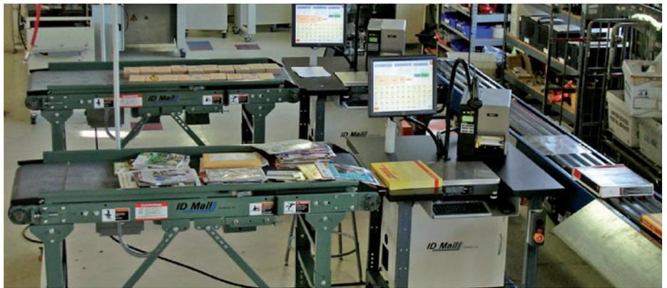
loading batches of items that automatically transfers them to the operator as pieces are processed. The MMW includes a Windows computer, industrial indicia label printer, postal certified weighing scale, barcode scanner and 17in touchscreen monitor, software and workstation.
