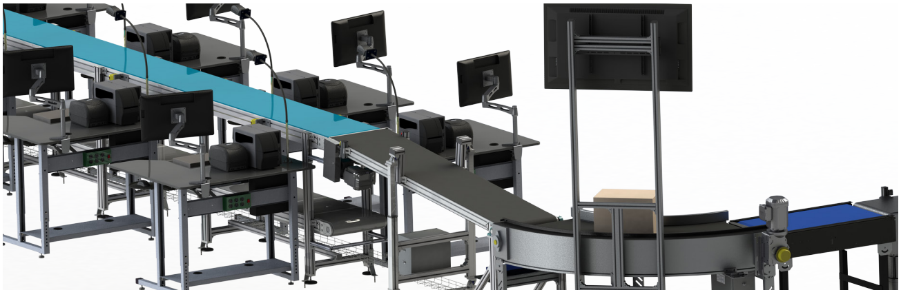
Over Under Conveyor Design for faster manual labeling and direct sorting when desired
